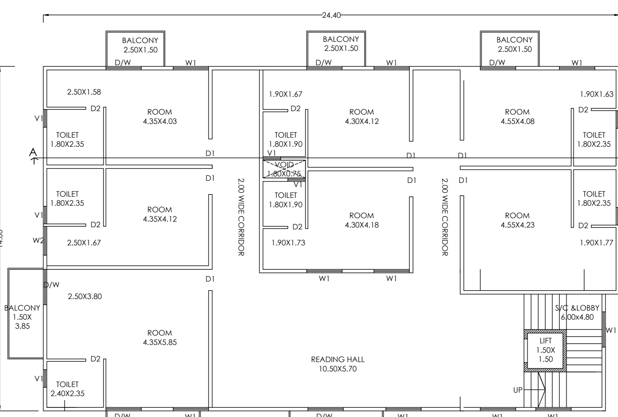
TYPICAL FLOOR PLAN (7X3 = 21 ROOMS) SECOND, THIRD & FOURTH FLOOR +6.29M ht +9.16M ht +12.03M ht.
